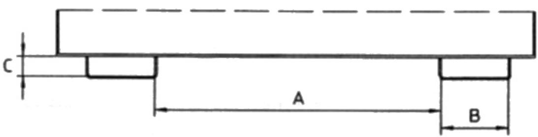
The diagram shows a side view of a container with a top flange. Dimension A is the length of the main body, B is the width of the base, and C is the height of the base. The top flange is shown with a dashed line indicating its position relative to the main body.
